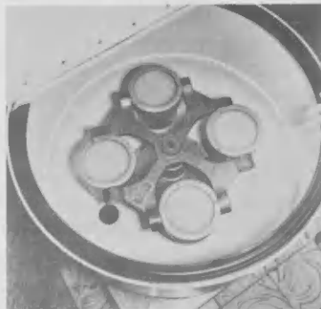
A centrifugal separator which separates the gel from crushed aloe leaves.
